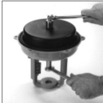
Fig 2 - Remove Stem Nut, and Washers
