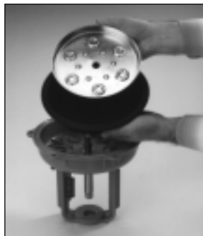
Fig 5 - Reverse Replacement of Diaphragm and Thrust Plate
