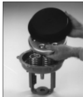
Fig 5 - Replace Springs, Reversed Thrust Plate and Diaphragm
