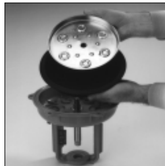
Fig 4 - Remove Thrust Plate and Old Diaphragm
