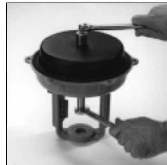
Fig 2B - Remove Stem Nut, & Washers
