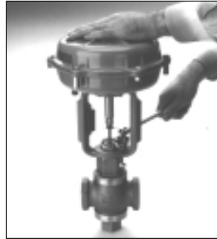
Fig 1 - Tighten the Bonnet Lock Nut on the Bonnet
