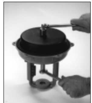
Fig 6 - Replace Washers, Tighten Stem Nut
