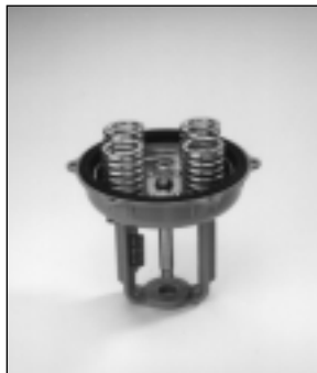
Fig 2A - Remove Upper Housing to Expose Springs
