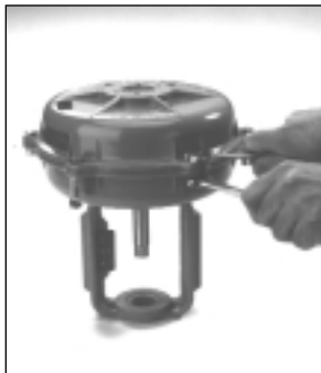
Fig 1 - Remove Housing Bolts
