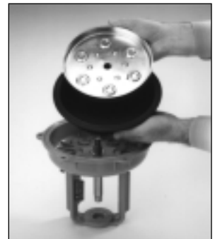
Fig 2C - Remove Washers, Thrust Plate, Diaphragm
