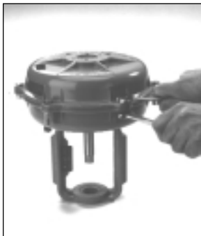
Fig 1 - Remove Housing Bolts
