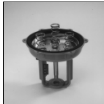
Fig 2- Remove Upper Housing
