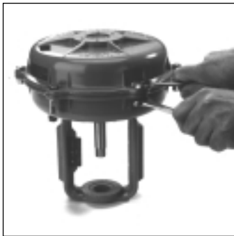
Fig 1 - Remove Housing Bolts
