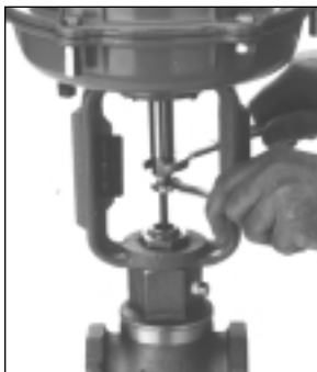
Fig 3 - Loosen Stem Locknuts
