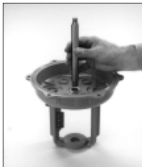
Fig 4 - Remove and Replace Stem
