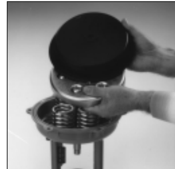
Fig 3 - Remove Diaphragm (Leave Thrust Plate On).
