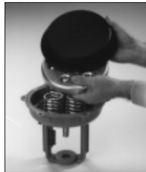
Fig 2B - Remove Diaphragm and Thrust Plate
